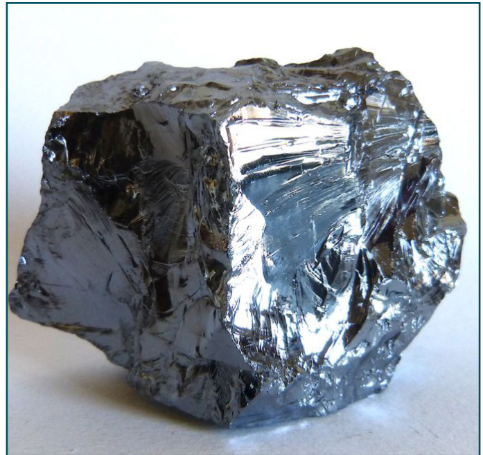
Silicon is a hard, brittle crystalline solid with a blue-grey metallic lustre
